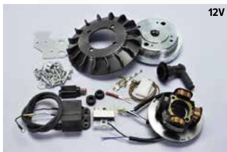
171.0543 Vespa 125 ET3 cone/cono Ø20, flywheel/volano 1,2Kg
