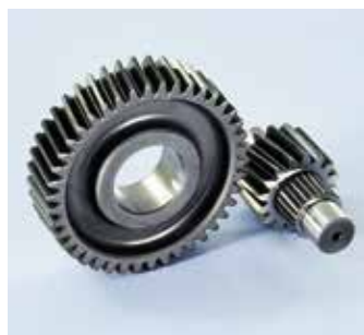
202.1416 Vespa 125/150 iGET Euro 4 Z=16-42 Secondary ratio-Secondario
